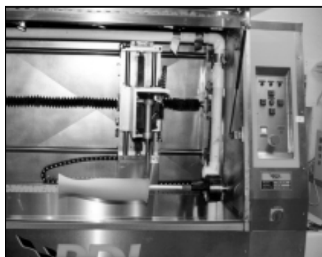
CAD-CAM carver shapes endoskeletal lower-limb foam cover. Courtesy Prosthetics Research Specialists.
